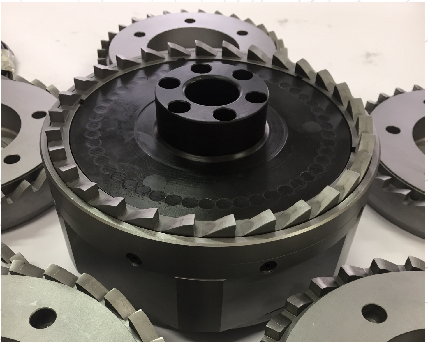
The special toothed clutch ESB-210/Z with the armatures
